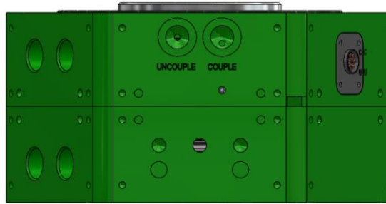
Figure 6.2-2. E125LP Tool Changer – Docked Position
