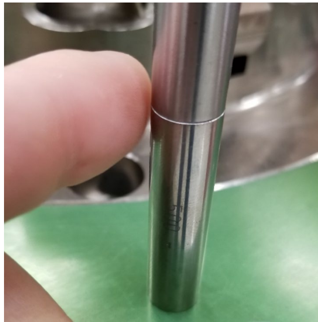
Figure 4.1-2. Concentricity of Teach Pins
